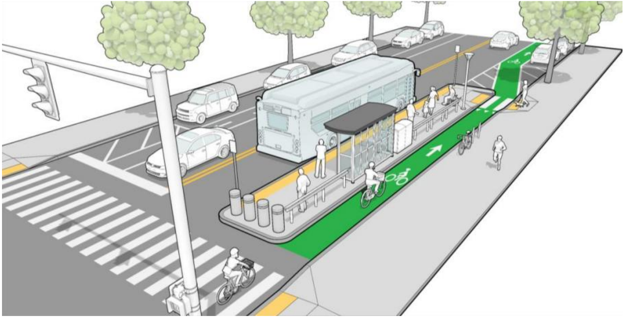
Figure 2 Floating Bus Stop Design (Toole Design Group, McMahon Transportations Engineers & Planners, RIPTA)
